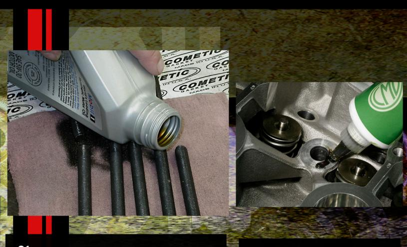
**51.** The stock head bolts are a torque-to-yield design, so they should not be reused. Use the new head bolts that come with the Head Gasket Kit (pn 12595961)—it also includes the head gasket, intake gasket and exhaust gasket.
