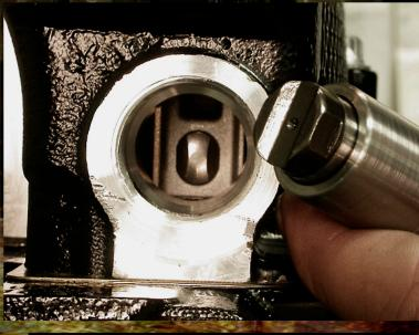
**92.**The black guide bolt access hole is now going to be closed up with this Allen plug. A 10 mm Allen wrench will be needed and some Loctite 567 thread sealer applied about two threads wide around the plug. Install about a ¼-turn past hand tight.
