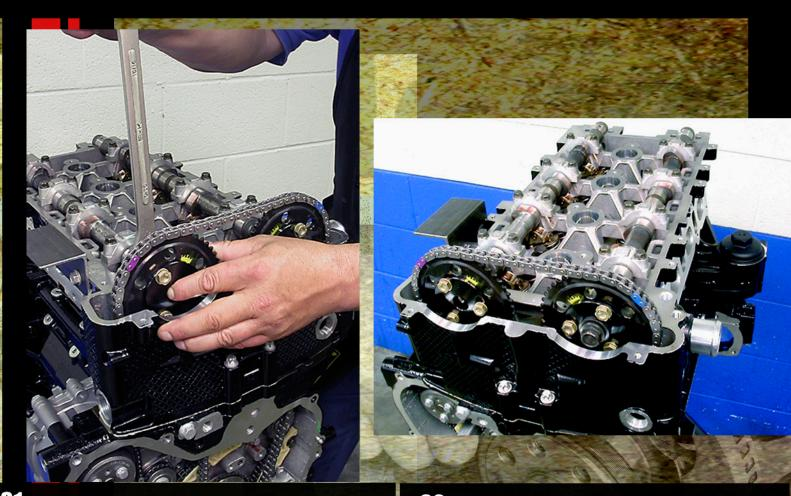
With the chain in the correct position (purple key on line) on the exhaust cam gear (marked with an 'E'), position it up against the front of the cam while slightly rotating the cam clockwise (from the front of the engine) with a 15/16-inch open end wrench to mate the slot in the cam to the gear. Hand tighten three 13 mm bolts and center 18 mm bolt until engine is timed (then torque to 65 ft-lb).
