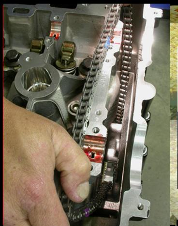
Turn the chain and maneuver past bumps into final position. Then, carefully rotate the chain 90 degrees while spreading it to out past two tight spots in the chain area. Be patient...the chain will fit between these two areas, but there is not a lot of room to maneuver it.
