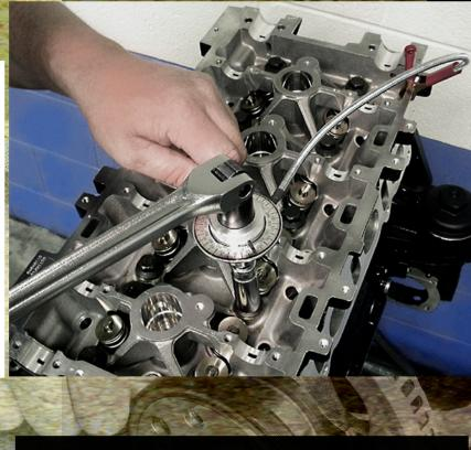
The head bolts then need to be 'twisted' another 155 degrees to complete the clamping down of the head on the block. Again, start with the center head bolts and work radially out towards each end of the head.
