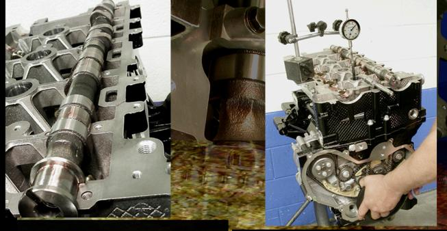
**75.** There is only one position the cam can be installed at where the lobes are not directly pushing on a follower—and you're looking at it. This simplifies the process of torquing the cam caps to 89 in-lbs (see caption 77 before doing the torquing) and reduces the chances of getting a component 'cocked' while doing the torquing.
