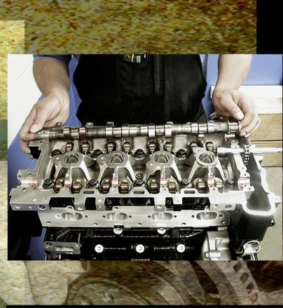
**14.** The factory camshafts are replaced with performance cams from Comp Cams. The intake cam needs to go in the engine first. A Comp intake cam with the following specs is being used: 0.441 inch net lift with 218 degree valve duration at 0.050 inch lift on 109 degree lobe separation. Apply engine assembly lube to the lobes and bearing faces before installing in the engine (see next caption for how to position cam in 'sweet spot').
