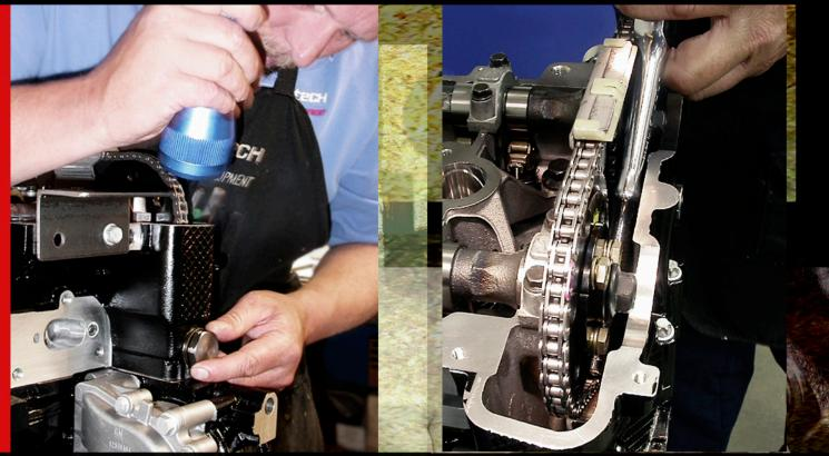
The slot and guide are aligned by inserting the tensioner piston assembly into its mounting hole and viewing the mating of these two components through the chain drive access in the top of the head. Use a flashlight to add light to the tight confines. Once these have mated, tighten down the threads on the piston tensioner (make sure to add the 567 thread sealer Loctite to the threads). Tighten to about a ¼ turn past hand tight.
