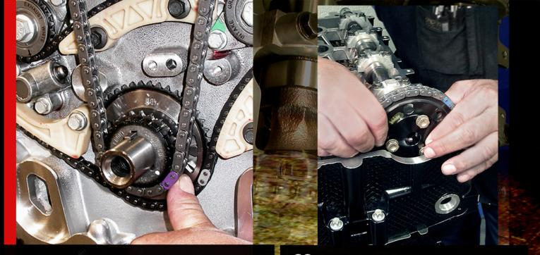
**79.** Now is the time to start positioning the cam drive chain by placing the crank gear with its arrow pointed in the 5 o-clock position and this purple colored link on the arrow.
