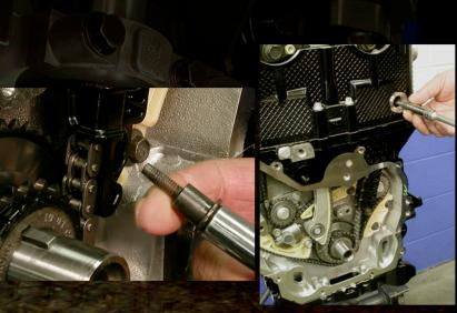
**86.** and **89.** To final install the black guide, apply one drop 277 red Loctite to the bolt threads and Torco on the face of the guide, make sure the floater shims are on the bolts and then install. Torque bolts to 89 in-lbs. *Note*: The top bolt is installed through an access hole in the block that has a plug to cover the hole (*shown in a later step*).
