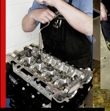
**63.** The bolts are long, so it will help if you use a speed wrench to get the bolts seated down onto head.
