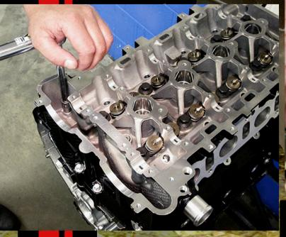
67. There are four E12 Torx 8 mm bolts at the front of the head that need to be torqued down (oil threads, lube backside of heads and torque) to 15 ft-lbs.
