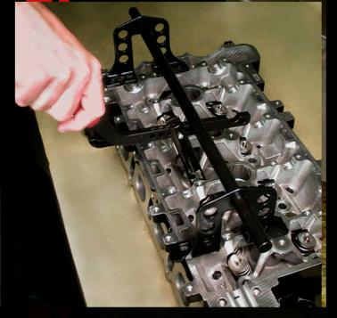
**43.**To change the valvesprings, this Goodson (Pn CF300) valvespring compressor should be used along with safety glasses. It consists of two stands and a round bar that allows a lever-action spring compressor to be used across the length of the head.
