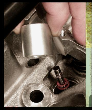
45. Before installing the performance valve-springs, you must check the 'installed height' with a height measuring gauge and spacer. On the Ecotec cylinder head, it is recommended a 1-inch spacer be used to minimize the struggle of maneuvering around the throat depth and tight confines of the head design. Make sure the valve stem seal is installed over the valve stem during this procedure, as its thickness is part of the 'installed height' measurement.
