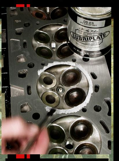
**53.** Then apply a light skim of grease around the perimeter of the chamber.
