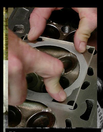
54. A lexan CC'ing cup is required to seal off the chamber volume. Press the cup firmly against the face of the head to seal it tightly to the grease.
