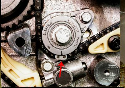
**35.** With the No. 1 piston at Top Dead Center (TDC) of the combustion stroke, begin to install the chain (*coat it with engine oil before installing*) to drive the balance shafts and water pump. We say 'begin' because the drive chain has colored links that need to mate with specific 'dots' on each gear—and this usually takes a few shots before you get it all correctly 'timed'. Put colored links on the arrows on the gears like this (*arrow*).
