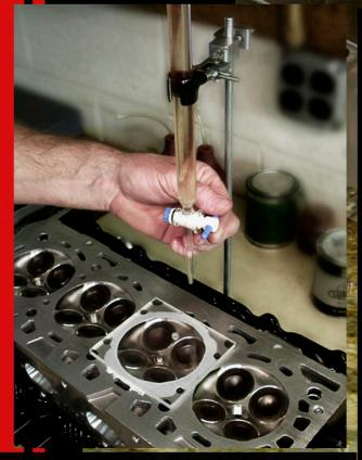
With a 100 cc burette filled to a measured level, pour fluid into the hole in the CC-cup until the chamber is filled. Read the new level on the burette—the change is the volume of the combustion chamber. Record this value for each chamber.
