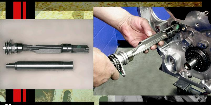
**33.** The stock balance shafts (top) are scalloped so when they spin, the forces generated by the movement of the internal components are offset to smooth the operation of the Ecotec engine. Racing-oriented engines aren't concerned with this 'comfort', so a tube (*bottom*) is installed to replicate the balance shaft, but not lose the 10 hp it takes to spin them.
