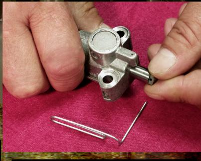
**36.** Now the chain tensioner needs to be 'set' in a relaxed state for installation. To begin this process, twist the piston 45 degrees to allow the plunger to be depressed.
