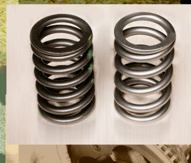
42. A set of performance valvesprings are installed at a 1.290-inch height and feature an 85 lb/in seat pressure and a 190 lb/in over the nose pressure. If you make a change to a performance cam, you must add performance valvesprings like these to maintain control of the valves during the engine operation.
