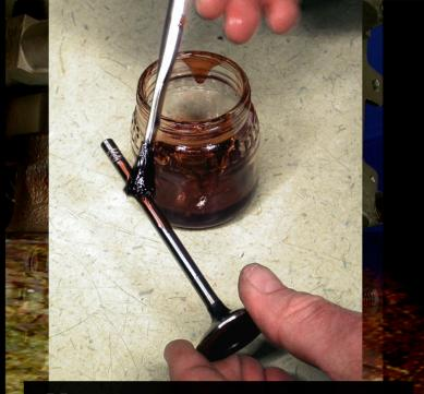
With the valves out, it's a good time to apply Torco engine assembly oil to the stem before sliding them back in the guides.
