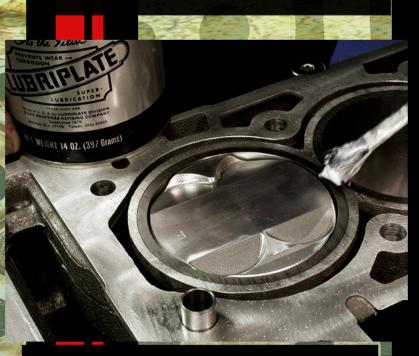
**57.** Apply a light coat of grease around the perimeter of the bore and install a CC-cup. In this case, a 65 cc Plexiglas CC-cup was used.
