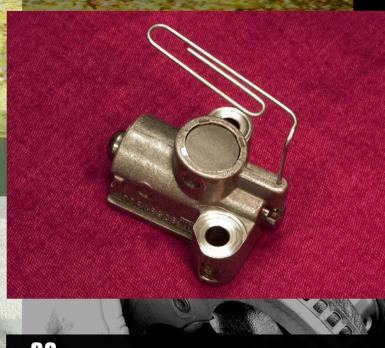
Using a paper clip that has been straightened, push the one end into the tensioner body/piston hole to hold the piston down until it's installed. There is a "tool" you can buy to do this.
