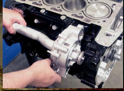
**32.**The water pump is installed from behind the front cover mount to the left of the crank. Three of the four bolts that thread in from the front of the engine should be installed now—the fourth is a long bolt that is installed after the cam chain drive and front cover is fully installed. Torque these bolts to 15 ft-lbs.
