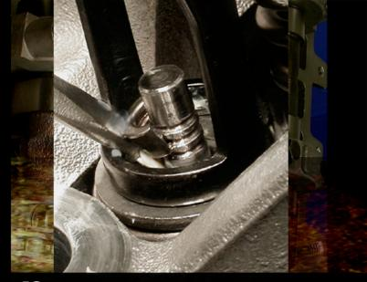
**48.** The Goodson universal OHC/DOHC valvespring compressor has been modified to mount to the Ecotec head bolts. Use it to compress the valvepring and push the 1st lock onto the stem of the valve.
