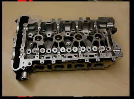
With sixteen valves, changing all the valvesprings on the Ecotec engine can take a little time. But now you know what tools are required and how to use them to accomplish this task. Whatever performance additions you make to the Ecotec, plan on upgrading the valvesprings to handle either the more aggressive cam or increased RPM.
