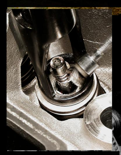
Put a new dab of white grease on the screwdriver and the second keeper on the grease to install it in the retainer. Compress the spring and slide the keeper into the three grooves on the valvestem to seat it completely. This can be tricky as the keepers on the Ecotec butt end-to-end to allow the valves to rotate—this is why it's so important to get the keepers properly seated in the retainer.
