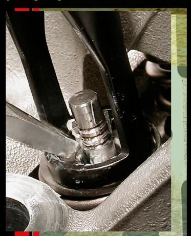
49. Once the first keeper is seated on the three grooves it sits in, use the screwdriver you installed it with to 'push' it around the backside of the valvespring retainer. This way, you can install the second keeper in the same opening.
