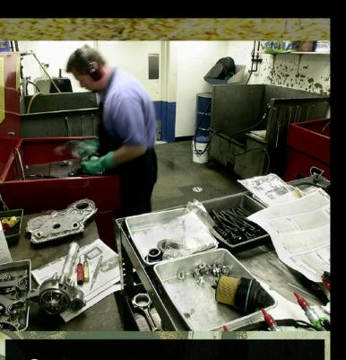
All the components need to be thoroughly washed in a solvent tank and blown off with compressed air (make sure there is a water separator in the air line to minimize the moisture in it) to insure the engine components are clean as they go together.
