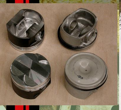
**10.** The stock eutectic cast aluminum pistons (*right*) are quality pieces for the 205 hp supercharged production engine, but once you start to move up in power production, aftermarket forged aluminum pistons are required to handle the rigors of big power. These pistons have a slightly higher piston height, which raises the compression ratio from the stock 9.5:1 to 10.0:1.
