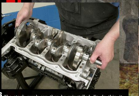
The stock crank can then be reinstalled. To do this, it should have been cleaned, measured and stored until the time came to install. Then, with the main bearing surfaces liberally coated with Torco assembly lube and the rear seal in place, the crank can be lowered into the top half of the engine block (with the block on an engine stand in the upside down position).
