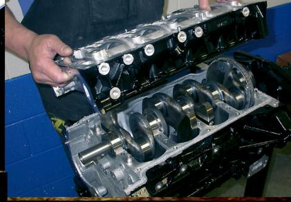
**21.** There are dowels that locate the engine main cap girdle on the block, so it needs to be carefully aligned and pushed on evenly. A little force will be required to seat the girdle on the dowels—it might help to carefully work the girdle back and forth on the dowels to get it fully seated.
