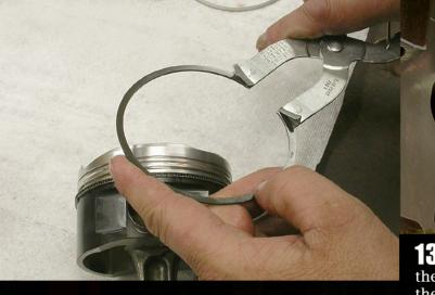
**12.** Using a ring spreader, carefully open the ring to install them in the ring lands of the aftermarket piston. These rings can be a little brittle during this step, so do not spread them any more than you have to—or you may break them
