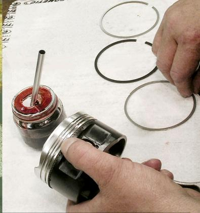
While the stock pistons need to be replaced, the stock rings are more than ready to handle big power. To install the rings in the forged pistons, start by wiping the rings off with a lacquer thinner soaked lint-free paper towel and then lightly lube the rings with engine oil (in this case 5W30 synthetic oil was used).
