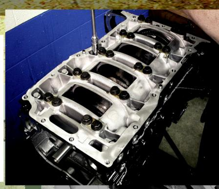
**27.** As the last step in assembling the bottom end of the engine, torque the oil pan rail bolts to 20 ft-lbs, install the oil pump pickup and install the cast oil pan, torquing the bolts to 10 ft-lbs.
