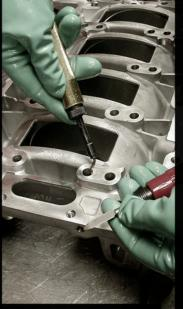
**1.** As an added level of insurance, some engine builders recommend lightly going over the deburred edges with a rotating abrasive wheel —like has been performed on the combustion chamber lip on the Ecotec head (see arrows). This step removes any metal that has been 'folded over' by the knife or machinists tool and requires EXTREMELY thorough cleaning in a wash tank afterwards to remove ALL of the abrasive debris from the engine—any of this abrasive will quickly destroy an engine.
