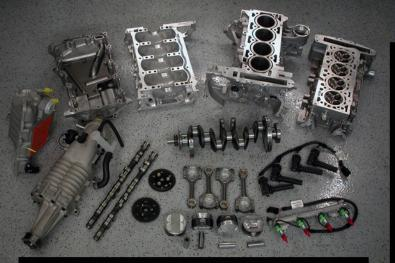
Most of the components used to build this engine are bone-stock—a testament to the capability of the production pieces. The aftermarket performance components needed to make this big power per Liter number (*like 150 hp/L*) include high flow fuel injectors, forged aluminum pistons, higher spring rate valvesprings, more aggressive camshafts and a new calibration and controller.
