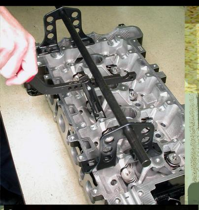
**2.** Once removed from the block, the cylinder head requires a few special tools, like this valvespring compressor assembly (*Goodson PN CF-300*), to tear down and then reassemble. This step the install of the performance valvesprings, which are needed to handle the more aggressive lobe profiles of the performance cams. For more details on this, check out the section on "Head Assembly" that will appear in the third installment in this series.
