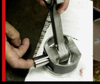
To install the aftermarket forged aluminum pistons on the stock rods (which are more than capable of handling 300+ hp), install a circlip on one side of the piston (to see how to do this, refer to the next caption). Then, wipe down the stock 2.0 L Ecotec pin with assembly lube and slide it into the piston pin bore. As a note, the stock pins received a 0.020 wide, 45-degree chamfer on the ends of the pins to increase the 'lock' on them.
