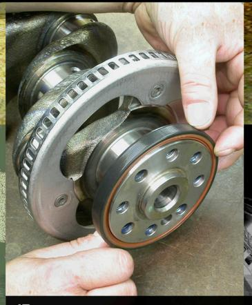
The rear seal is an O-ring-style piece that should be seated on the crank (like this) before the crank is installed in the engine block. Wipe the crank seal surface with a light coat of Torco engine assembly lube before sliding the seal into position.
