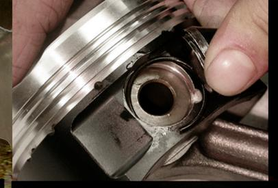
**9.** To lock the piston pin in place, install the second 'circlip' in the forged aluminum piston. The best way to do this is to seat one end of the circlip in the piston pin circlip groove while holding the circlip close to the piston with the finger on one hand and push on the other open end of the circlip with a large, flat metal dowel with your other hand until the end of the circlip snaps into place in the piston groove.
