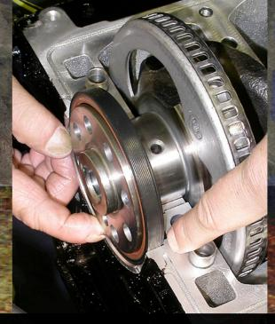
17. With the crank seated in the engine block, the rear seal should pushed up against the engine block sealing face. Do this around the circumference of the block material.
