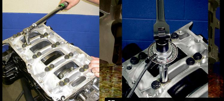
**24.** The girdle bolts are all torqued to 15 ft-lbs starting with the center bolts and moving radially outward to the bolts at either end of the girdle. (see torque sequence illustration below)
