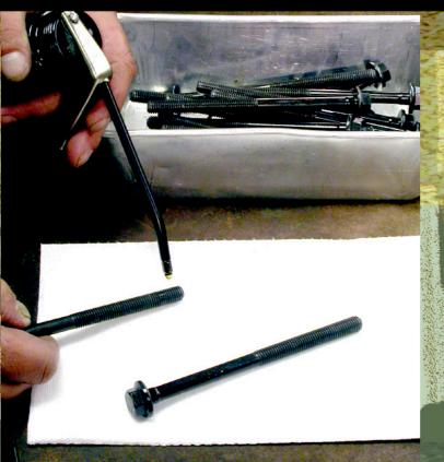
**22.** The fasteners for the main girdle are what GM calls 'torque to yield'—which means they stretch beyond a reusable limit to provide consistent clamping force through multiple situations. You'll need to buy a new set (GM pn 11519783) when building this engine (along with a set of head bolts shown in caption 64 in the next installment). Apply engine oil to the threads of the bolts.
