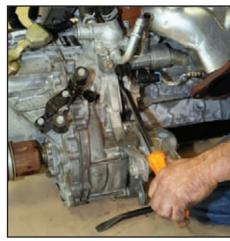
Start by wedging a "pry bar" into the space between the engine case and the transmission mounting flange on the exhaust side of the engine. Lightly pry it apart a few millimeters—if this takes more than a few tugs to release the two, recheck your work. You probably missed a fastener, as this shouldn't take an enormous amount of force. Stop and move to the other side of the engine to slowly work the transmission off evenly.
