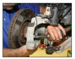
To begin the reassembly of the front suspension/drivetrain, start by pulling the wheel hub out slightly to position the axle splines behind the hub. Align the splines of drive axle with those in the drive hub ...
