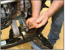
Tighten the bolt to 1/4-turn past hand tight before torquing to 74 ft-lbs (100 N-m).
