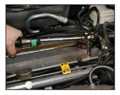
Hand start the threads on the 10 mm hold-down bolt for the fuel rail and torque to 89 inlbs (10 N-m).
