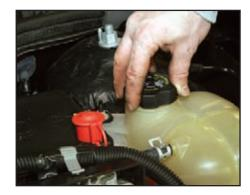
Hand tighten the coolant tank cap.
