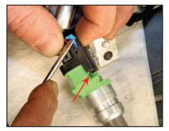
Each electrical connector has a blue safety lock that needs to be pulled up, as shown, before the electrical connector release tab can be depressed (in the direction of the red arrow) to release the electrical connector.
