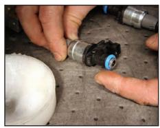
Very carefully wipe a light coat of Vaseline onto the O-rings of each injector.
