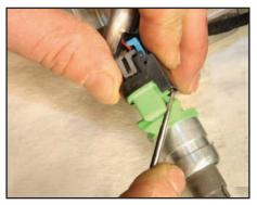
Depress the lock on the electrical connector and pull the electrical connector off each injector by gently wiggling and pulling on the connector and injectors until they come apart.
