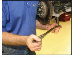
Torque the tie rod end nut to 18 ft-lb (40 N-m) and then rotate the nut another 90 degrees.
