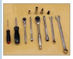
The tools required to install the Stage 1 and Stage 2 performance upgrade kits include: a small flat screwdriver, 1/2-inch and 3/8-inch ratchets and extensions, various sockets
