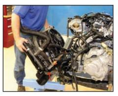
Start by positioning the radiator/condenser/intercooler/fan assembly up on the engine cradle mount at the front of the engine cradle. There are two rubber bushings on the assembly that seat in two holes on the cradle (arrow on one)—so make sure these are in place before proceeding.
