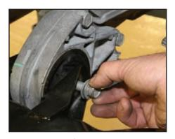
Install the 18 mm front engine mount bushing bolt and hand start the threads.
