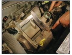
It is a good idea to make sure the supercharger bypass seal is still in place on the intake manifold (right hand pointing to it) and that the metal guide pins are installed in the intake before going on to the next step (left hand).
