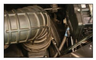
The supercharger removal starts with removing the inlet duct that connects the air cleaner to the throttle body. On the Cobalt, this requires loosening two 8 mm hose clamps at each end of the hose; the lon has 7 mm bolts on these clamps.
