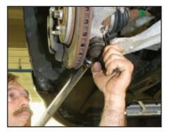
Torque the ball joint bolt and nut combo to 41 ft-lb (55 N-m).
