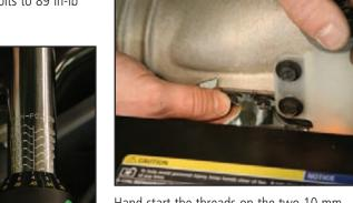
Hand start the threads on the two 10 mm bolts that hold the intercooler reservoir onto the supercharger housing and torque the bolts to 89 in-lb (10 N-m).
