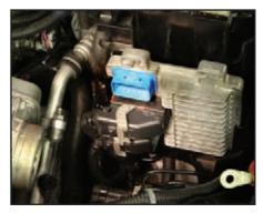
Install the "black" connector next in the middle receptacle by pushing the connector on and pivoting the lock tang over.
