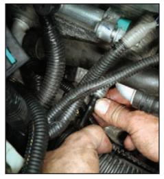
Install the dry break fitting for the clutch slave system by pushing it firmly into the machined distribution block mounted on the top of the transmission.
