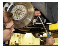
Torque the U-joint lock nut to 25 ft-lb (34 N-m).
