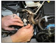
Install the vacuum line onto the bypass solenoid.
