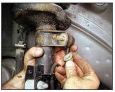
Hand start the 18 mm swaybar mount nut on the threads of the swaybar throughbolt.
