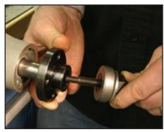
With the blower on a bench, situate the Stage 2 mounting hub with the deep shoulder toward the outer edge of the shaft. The Stage 2 pulley mounts to this hub.
