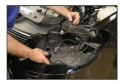
Hand start the threads on one of the three 10 mm headlight closeout bolts. You'll probably need to wiggle the closeout panel a little to get the holes to line up.
