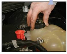
Tighten the cap back onto the coolant reservoir.
