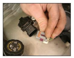
Remove the map sensor electrical connector by lifting the lock tab and pulling connector off the blower housing.
