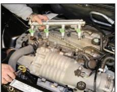
Now is a good time to inspect the fuel line fitting to make sure the green plastic washer and blue O-ring are seated in the fuel rail (these usually are nested into this position and will not come out, but it's a good idea to make sure they are there before proceeding).
