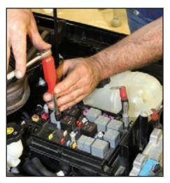
Hand start the two 10 mm bolts used to fasten the midplate on the baseplate of the fuse
