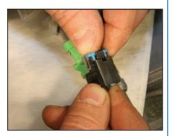
Push the blue safety lock back down after the injector has been removed from the connector in preparation for reinstalling the connector.
