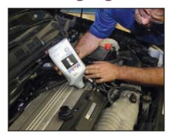
Check the dipstick and top off the oil in the engine w/ Mobil 1 synthetic oil (a factory-fill oil).
