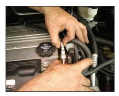
To check the "lock" of the fittings, lightly pull the two fuel lines apart—if they stay together, you are locked in place. If they separate unevenly, you need to push them together more firmly.
