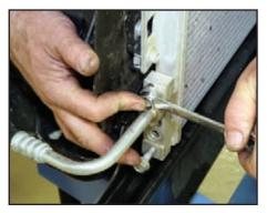
Tighten the 13 mm holddown bolt for the A/C fitting to 12 ft-lbs (16 N-m).
