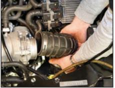
Reinstall the air cleaner to supercharger induction tube and tighten the two hose clamps to 89 in-lbs (10 N-m).
