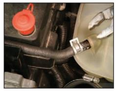
Use pliers to compress the clamp tangs, slide the hose on the nipple of the overflow tank and release the clamp to hold the hose on the tank.
