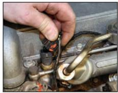
Reinstall the temperature sender electrical connector onto the sender by pushing it on until the lock clip clicks into place.
