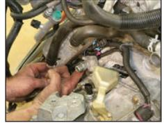
Fish the speed sensor connector and reverse lights connector wiring looms through this same area (it's tight, so be patient!) behind the machined fitting. (Note for 2004 MY Saturn Ion RL owners: the speed sensor tone wheel is mounted on the axle shaft. The sensor is mounted on brackets at this location).
