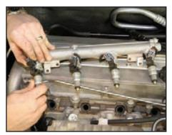
Apply a light coat of vaseline to the injector O-rings and install the Stage 2 fuel injectors onto the fuel rail (for more detail on this, see the Stage 1 injector install). Position the fuel rail over the engine with the fuel fitting on the passenger's side and install the electrical wiring onto each injector (for more on this, see the Stage 1 install).
