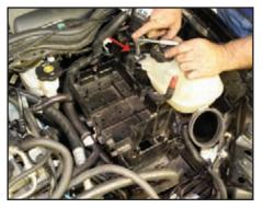
Fasten the baseplate with the two 13 mm bolts and one 10 mm nuts. Torque these to 89 in-lbs (10 N-m).
