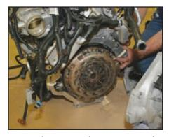
To start, the engine and transmission need to be bolted together. This begins with the positioning of the factory engine-to-trans shim on the pins of the engine bellhousing.
