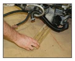
A great trick to make this job easier is to have a bunch of different thickness wood pieces available, like this 1x3 wood block, to shim the engine and transmission in the front, back and sides to hold the pieces level as everything gets closer together.
