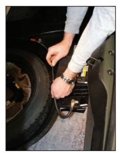
Reconnect the negative battery cable and torque to the cable end nut to 89 in-lbs (10 N-m).
