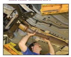
Slide the "downpipe" into position in the vehicle and hand start a few of the fasteners to the rear portion of the exhaust.
