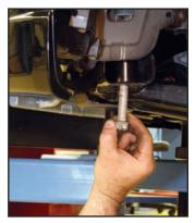
The cradle body hole is very close in diameter to the bolt, so the cradle and body need to be very close in alignment for the bolt to go up into the threaded body hole. Hand start the threads on the four 21 mm cradle/body mount bolts.
