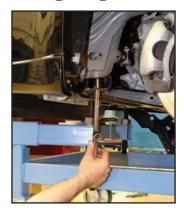
The engine cradle will most likely need to be "coerced" slightly with an awl slid through the cradle bolt and body holes. To do this, once the awl is fully seated in the holes, pry the cradle in the direction required to line the holes up.
