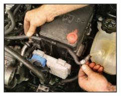
Position the radiator coolant overflow tank vent tube across the fuse box cover and seat it in the two plastic tangs in the cover.
