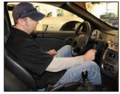
Turn the key to on to cycle the fuel pump and pressurize the fuel rail. If inspection of fuel system shows no leaks, start vehicle and reinspect under the hood.
