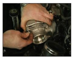
Install the throttle body on the supercharger flange and hand start the threads on the four 10 mm bolts.
