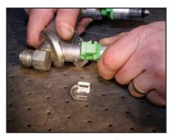
With the retaining clip pulled off, wiggle each stock injector out of its seat on the fuel rail.
