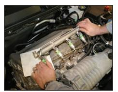
Remove the two 10 mm bolts holding the fuel injector rail onto the engine and pull up on the rail while slightly wiggling it. Once off, disconnect the fuel injector wiring. For more on this step, see the section titled "Removing Electrical Connector Detail on Fuel Injector" in the Stage 1 install section.
