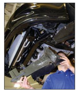
Position the driver's side splash panel up in the front of the engine cradle. Locate the holes in the panel with the many pushpin and screw holes in the vehicle.
