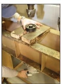
With the supercharger unbolted from the vehicle, it can be placed in the press with the pulley captured by press plate anchor points on the hydraulic press. The supercharger will actually be hanging by the pulley as the press pushes the supercharger main shaft out of the stock pulley.
