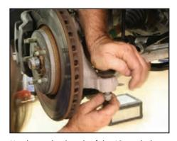
Hand start the threads of the 18 mm lock nut.
