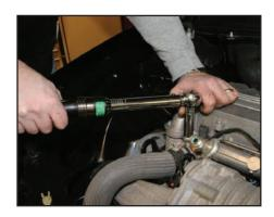
Torque the steam pipe bolt to 89 in-lbs (10 N-m).
