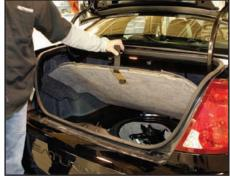
Move to the trunk to disconnect the negative battery cable from the battery. Start by lifting the carpet liner off the battery.
