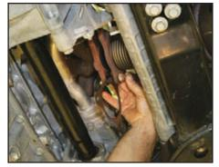
Use one of the three exhaust-header-to-downpipe bolt/studs to position the gasket in place. Then, rotate the gasket into position between the header and downpipe and install the second bolt/stud.
