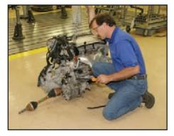
With all the engine-to-transmission bolts now removed, the process of separating the transmission case from the engine block is next.
