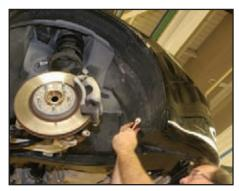
Reinstall the black plastic "splash panel" on the passenger's side of the front fascia by positioning it in place and installing the many pushpins and two 7 mm bolt screws.
