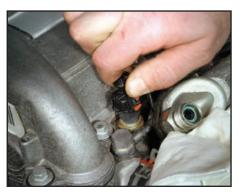
Unplug the coolant temperature sender electrical connector from the front of the engine by pushing on the black plastic tang with your thumb while carefully pulling up on the connector.
