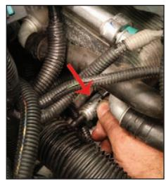
Push the "C" clip into the machined clutch slave system distribution block to lock the dry break in place on it.
