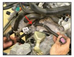
A major trunk of the wiring harness needs to be routed behind this machined fitting (arrow) because it is just long enough to reach the various connectors it attaches to if routed through the area (we learned this the hard way!). Start by fishing the harness section through with this engine-to-body harness connector.
