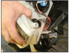
Feed the headlight wiring back into the closeout bracket as the headlight is brought closer to the headlight mount.
