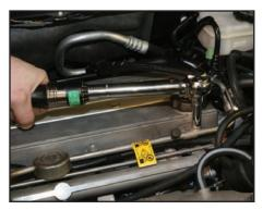
Hand start the threads on the 10 mm fuel line bolt, then torque it to 89 in-lbs (10 N-m).
