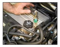
Pull the rubber plug you had in the fuel line in preparation for reinstalling it on the engine fuel line. Be careful to not damage the inner tangs on the dry break fitting when pulling the plug.
