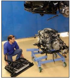
Roll the engine/trans/cradle cart under the engine bay of the vehicle up on the four-point lift. You will now be installing the radiator/A/C condenser/inlet intercooler system on the engine cradle.
