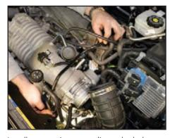
Install evaporative system line at both the controller and supercharger housing (see steps in the Stage 1 Install for details of how they were removed) by pushing the connectors over the mounting nipples.
