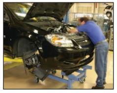
Basically, you need to be looking in the engine bay and from under the vehicle at every angle and corner to make sure the entire package is going in the vehicle without causing any damage, and lining up properly with the mounting holes for the engine cradle bolts.
