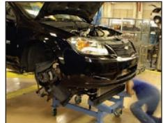
Check under the vehicle often to make sure all the wires, hoses and other equipment are not being damaged by crushing, scraping or other interference with the body as you bump the vehicle down very slowly.
