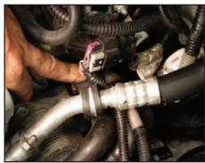
Push the black plastic pushpin on the A/C line down into this bracket on the engine to hold the hose in place.
