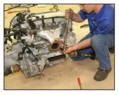
Torque the jackshaft engine block mount bolts to 37 ft-lb (50 N-m) in a radial pattern.
