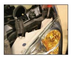
Hand start the threads on the two 10 mm headlight bolts and then tighten them to 89 in-lb (10 N-m).
