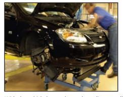
With the vehicle lowered past the radiator, you'll need to reach down into the engine bay to pull the wiring up out of the way of the engine mounts and engine bay sheetmetal.
