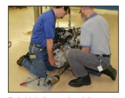
The bolt hole diameters through the transmission are tight to the bolts, so you'll need to have one person holding the transmission case tightly to the flange of the bellhousing, while the other person feeds the bolts through the transmission to get them started on the threads.
