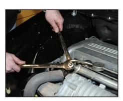
Torque the fuel line fitting to 124 in-lbs (14 N-m).
