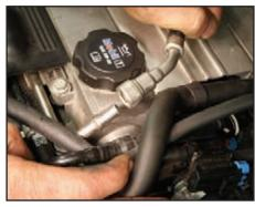
Firmly push the two ends of the fuel line together until you hear a very light "click" of the tangs locking in place.
