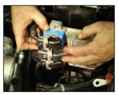
Install the "blue" connector in the top receptacle of the PCM and lock in place.
