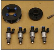
The Stage 2 upgrade kit for the LSJ Ecotec is a true step up from the Stage 1 kit. The Stage 2 adds a specially designed blower pulley and belt, and a powertrain control calibration that takes advantage of the increased boost generated by the smaller Stage 2 blower pulley.
