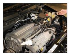
Remove the 10 mm bolt holding the fuel line onto the engine and pivot the fuel line off the front of the engine and lay it on the driver's side of the engine bay. This is required to access the fuel rail and fuel injectors, and remove them.
