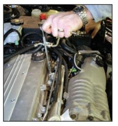
Remove the two 10 mm bolts holding the fuel rail in place on the engine. Note the location of the wiring and hoses in this area so you can reinstall everything where it needs to go during reinstallation.
