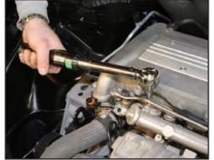
Hand start the threads on the fuel rail holddown bolts and then torque to 89 in-lbs (10 N-m).
