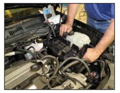
Push the many wiring connectors out of the area where the engine bay mounted fuse box baseplate is installed on the driver's side area of the engine bay. Then, lower the baseplate down into the area. Focus on locating the baseplate so the slotted opening goes over the bolt in the framerail and that the studs seat in the many holes located on the baseplate.
