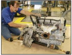
With the engine and transmission separation started, you can move to the end of the transmission and work it off the engine. Expect the engine and transmission to rock in opposite directions as they come apart, as they don't have "flat" bottoms—so watch the placement of your fingers!
