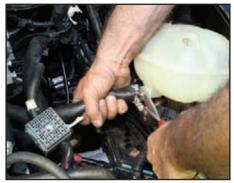
Compress the clamp on the overflow tank hose to allow the hose to be pushed onto the nipple on the overflow tank. Release the clamp to lock the hose in place.
