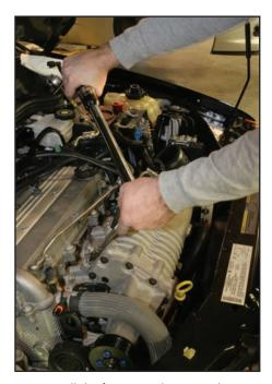
Now, install the four 6 mm hex supercharger bolts to intake manifold bolts and torque them to 18 ft-lb (25 N-m).
