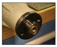
This is what an installed Stage 2 hub will look like on the supercharger shaft.
