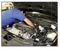
Reach between the engine and firewall to install the heater hose.
