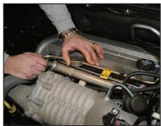
Apply a light coat of petroleum jelly to the mating surface of the fuel line fitting end. Position the fuel line and fitting together and hand start the threads on it.
