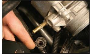
Remove the vacuum hose for the EVAP purge line from the nipple on the throttle body by rotating tab downward on the fitting to unlock the fitting and gently pulling it off.
