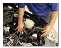
Install and route the boost control hose between the inlet portion of the supercharger and the control solenoid located on the driver's side of the cylinder head.
