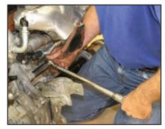
Using a deepwell 18 mm socket, tighten all eight transmission bolts to just past hand tight, then using a torque wrench (as shown here), tighten the bolts to 55 ft-lb (75 N-m) working on them in a radial pattern.
