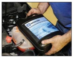
Add coolant to the fill tank. Be prepared: once the engine starts, you'll need to add coolant a few times until the system "burps" out all of the air and the coolant system is filled completely with a 50/50 mix of DexCool/water.
