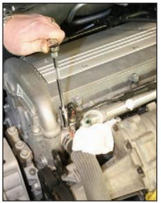
Remove the steam line fitting with 14 mm socket.
