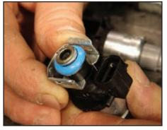
If they are not already on there, install the holddown clips on each of the four Stage 1 injectors. Make sure the open end of the clip is facing the electrical connector.
