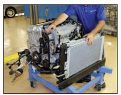
With the cooling system installed, the engine/transmission combination on the cradle is now ready to have the vehicle lowered down onto it.
