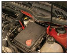
Start the install of the Stage 2 upgrade kit by locating the fuse block—in this case, this is a Chevy Cobalt SS Supercharged fuse block located under the hood. (for accessing the lon Red Line fuse block, see the beginning of this chapter in the Stage 1 install section).
