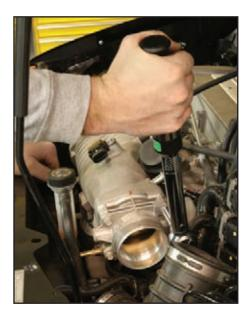
(Left) Torque throttle body bolts to 89 in-lb (10 N-m) in a radial pattern.
