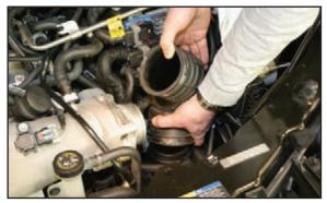
Pull the hose up off the air cleaner flange and out of the vehicle like this.
