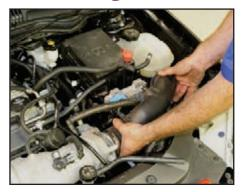
Install the inlet tube between the airbox and throttle body (mounted on the supercharger) by lowering the air cleaner end down into the engine bay and mating up the other end with the throttle body.
