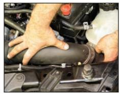
Slide the inlet tube inside the rubber hoses at each end of the tube.
