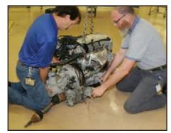
When mating the transmission up to the engine, you'll want to ask for some help, as the bottom of both the engine and trans are not even close to where the engine and trans need to be positioned to get them to mate to each other. To start, have your helper hold the passenger-side jack shaft and mount in position as the trans is slid into the proximity of the engine.
