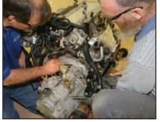
With at least one bolt hand started to hold the engine and transmission together, hand thread the remaining 18 mm transmission bolts in place
