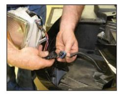
With the headlight bezel in your hand, plug in the electrical connector (make sure the lock tang 'clicks' into place).
