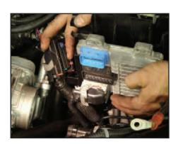
Begin installing the underhood wiring connectors by pushing the gray connector into the lower receptacle of the PCM and pulling the lock tang over to fasten the connector in place. NOTE: Fully seat the PCM connector before pulling the lock lever. Using the lever to seat the connector can cause the pins to expand, causing electrical issues down the line.
