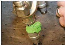
Note the "clocking" of the injector and retaining clip mounted on the fuel rail—install the Stage 1 injectors in this orientation. Use a screwdriver to lightly pry the injector retaining clips off each injector. These can be reused or the Stage 1 clips that come loaded on the injectors can be used.
