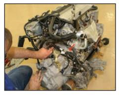
Pull the remaining portion of the wiring harness section through until it is lying on the transmission like this.
