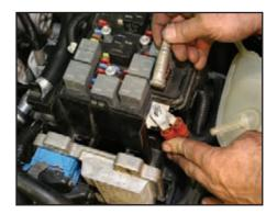
Position the two positive battery cables on the front corner of the fuse box and hand start the threads of the tall nut on the fuse box stud.
