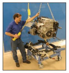
With the engine/trans and cradle positioned as shown here, lower the engine/trans down onto the cradle until the engine mounts slide into the brackets on the cradle.
