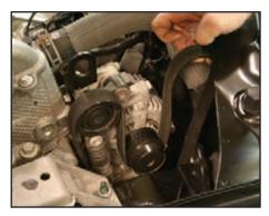
Once the belt is on the crank pulley, loop Stage 2 belt over the tensioner pulley and under the alternator pulley in preparation for looping the belt over the blower pulley when it is installed.
