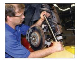
Torque the swaybar rod end nut end to 48 ft-lb (65 N-m).
