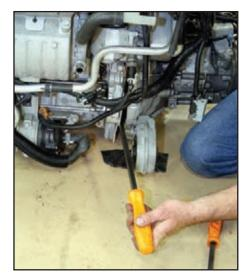
On the front of the engine, repeat the wedging of the pry bar and light tugging to separate the engine and transmission.
