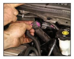
Attach this engine mounted body-to-engine electrical connector to the end mounted to the cowl of the Cobalt SS. Push the two connectors together until the lock tang "clicks."
