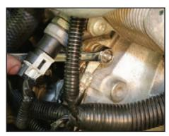
Install this main ground cable onto the stud/bolt of the transmission (there are two of these—one here and the other just above it) and tighten the 13 mm nut over it.
