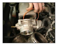
As you remove the throttle body, capture the red O-ring that seals the throttle body to blower and place it in a safe location for reuse. Place the throttle body off to the side in the engine bay.
