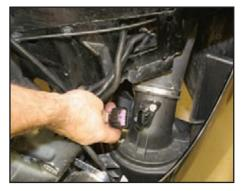
Reinstall the Mass Air Flow electrical connector on the sensor under the driver's side headlight area.
