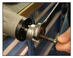
There are a few ways to install the Stage 2 pulley hub. One way is to use a power steering pulley installer with a 8 mm x 1.25 pitch threaded rod to thread into shaft (Kentmore P/N J-38823). With this unit, you thread the installer through the pulley hub and into the internal threads on the supercharger shaft before tightening the installer down until the Stage 2 hub sits flush with the end of the supercharger shaft.
