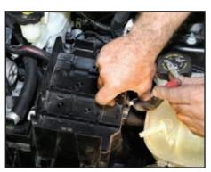
Feed the red power cable up around the driver's side of the fuse box baseplate in preparation for installing the cable on the front corner of the fuse box.
