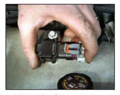
Push the MAP (manifold air pressure) sensor electrical connector onto the MAP sensor.
