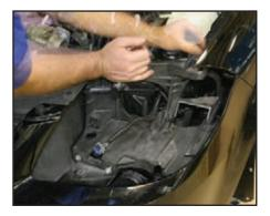
Hand start the threads on the second 10 mm mounting bolt while positioning the closeout bracket to line up the holes.
