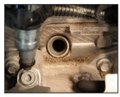
Make sure the factory fuel injector spacers are properly located in their bores in the cylinder head.
