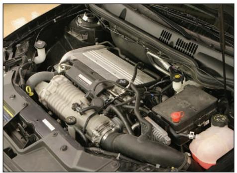
This is what the Ecotec 2.0 L LSJ engine and 5-speed transmission will look like when completely reinstalled in the Chevy Cobalt SS.
