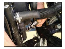
Install the lower hose for the inlet intercooler system by pushing the hose on the fitting, compressing the clamp and positioning it in place before releasing clamp.
