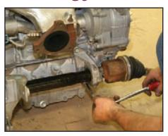
Hand start the 15 mm bolts for the jackshaft engine block mounts. Then, using a deepwell 15 mm socket, tighten these bolts to just beyond hand tight.
