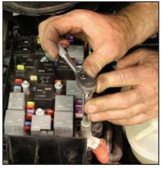
Hand tighten the tall nut and torque the nut to 89 in-lb (10 N-m).
