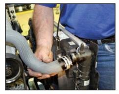
Install the passenger side radiator hose on the radiator fitting by compressing the clamp, sliding the hose in place and releasing the clamp to lock it on the fitting.
