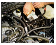
Continue positioning wiring connectors on the baseplate until it is filled with connectors seated in their respective areas.
