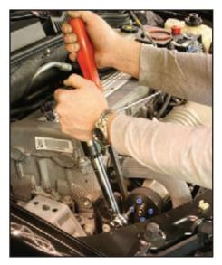
Now with the belt holding the pulley tightly, and a pry bar wedged against the pulley, torque the four custom Stage 2 bolts to 16 ft-lb (22 N-m) in radial pattern using the Stage 2 tool in 8 mm socket.
