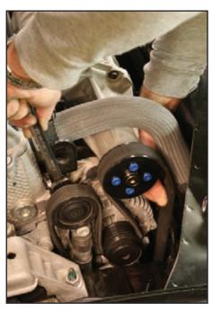
Here is what the Stage 2 belt should look like at final installation. As a precaution, inspect all pulley/belt interfaces to make sure the belt is properly seated on the pulleys before moving on to the next step.
