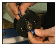
Next, the Stage 2 pulley is positioned on the Stage 2 hub and the Stage 2-provided fasteners carefully threaded through the pulley and into the hub. Be careful getting these started properly on the threads as these are a tight interface!
