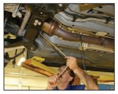
Torque the three bolt/studs at the header/downpipe flange to 22 ft-lb (30 N-m).
