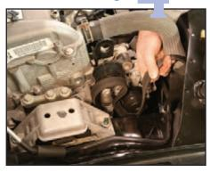
Now is the time to remove the stock front drive belt off the engine. This mostly requires lightly wiggling to get it off the crank pulley and out from between the body and engine.
