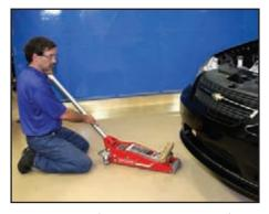
Use a hydraulic floor jack with a piece of wood on the lift point to jack up the passenger's side of the engine to get the upper engine mount on the passenger's side to line up with the engine mount. The photo at right shows where to lift on the engine oil pan.
