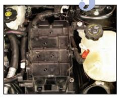
This is the baseplate fully installed in the vehicle. There will be five wiring connectors nested into this baseplate for the Cobalt SS, and three on the lon, that are sandwiched by the midplate to create the fuse box.
