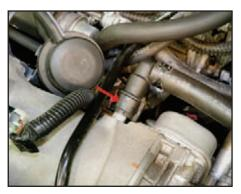
Push one end of the brake booster hose end onto this metal nipple (photo at left, arrow) located on the supercharger. Once the hose end is on the nipple (middle photo), push the lock tab down to affix the hose onto the nipple (arrow on photo on right). To test the lock, lightly pull back on the hose—it should stay in place.
