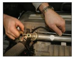
Hand start the threads on the steam pipe bolt after positioning the brass washer between the steam pipe flange and the cylinder head.
