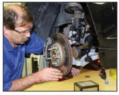
... And push the hub inward until the drive axle pokes out the front of the drive hub.
