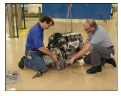
After getting the transmission case muscled up close to the engine bellhousing, start to line up the two locating pins and holes in the transmission case. These will help to guide everything together.
