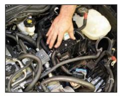
Position each wiring connector over the baseplate and seat it in the proper opening. Each connector will only fit in one opening on the baseplate—so don't force them! This might take some reworking of the wiring to get everything to fit properly.
