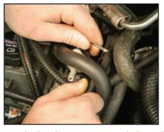
Use a hook tool to assist in getting the bypass hose to slide off the nipple of the boost bypass solenoid near driver's side of cylinder head of engine.
