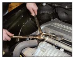
Torque the fuel line fitting to 124 in-lb (14 N-m) with 24 mm and 21 mm wrenches.
