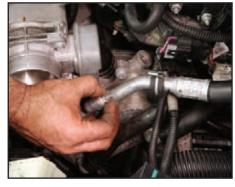
Wipe a light coat of Vaseline on the A/C line rubber O-ring and push the two fittings together. Hand start the threads on the 13 mm bolt that holds these two fittings together.
