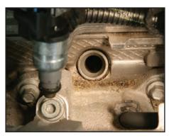
Make sure the plastic fuel injector spacers that rest in the cylinder head are fully seated by pushing down on them with your finger.
