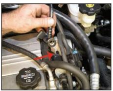
Push this canister purge line onto the metal nipple (arrow) until the lock "clicks."
