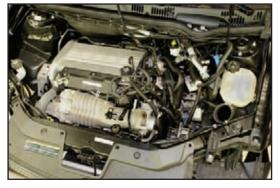
This is what the engine/transmission combination should look like when the body is fully lowered down on the cradle.
