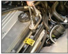
Remove 10 mm bolt holding fuel rail onto engine.
