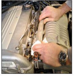
Wiggle and pull the fuel rail and fuel injector assembly out of the cylinder head. This should require minimal force. Be very careful—pull up in line with the fuel injectors to avoid causing any damage to the injectors. Tilt the fuel rail to drain any remaining fuel onto a rag before removing from the engine.
