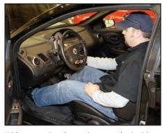
Without starting the engine, turn the ignition key to the "ON" position for the vehicle—this will intiate the fuel pump to run for a few seconds to pressurize the fuel rail. Wait about 10 seconds and turn key off and then back on. Do this sequence three times before moving to the next step.
