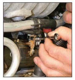
Install the small connector ignition switch wire onto the small stud and tighten the 8 mm nut to 1/8-turn past hand tight.
