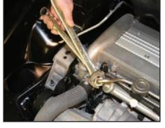
Loosen the 24 mm fuel line nut by pulling against a 21 mm open end wrench situated on the fuel rail anchor nut. This is to avoid twisting and possibly damaging the fuel rail as you apply torque to loosen the fuel line nut. Read the next caption before loosening the nut ...
