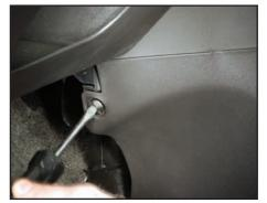
Start accessing the Ion Red Line panel by removing a standard screw from the driver side of the center stack.
