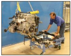
Lift the engine/trans combination up with a chain attached to the two factory engine lift brackets and slide a cart with the engine cradle on it under the engine/trans. As we said in the previous chapter, this cart is custom built for these installs, but a moving cart with some blocks of wood nailed to it to stabilize the cradle will work.
