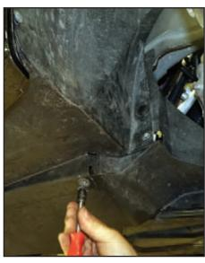
It helps if you have a pushpin with you so you can push one in place to hold the panel while you install the remaining five pushpins and four 7 mm bolt screws in both panels.
