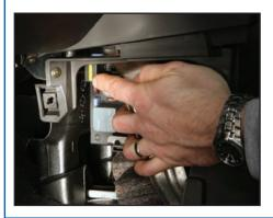
The Red Line fuel pump relay has a yellow stripe on it and is located in the upper left corner of the fuse block (finger pointing to it on left). Reach in and pull the relay out at this time (right).
