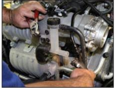
Install the upper intercooler hose on the plastic fill assembly by compressing the clamp with pliers, sliding the hose on the fitting and releasing the clamp.
