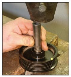
A shaft arbor extension needs to be used to allow the press to push the blower shaft out of stock pulley. Some enthusiasts have used a 13 mm or smaller deepwell impact socket as this spacer, but a dedicated arbor is recommended.
