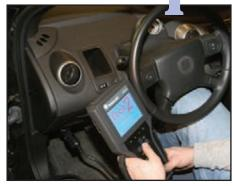
Now is the time to take your Stage 2-parts equipped vehicle to a GM dealer to have appropriate performance calibration flashed into vehicle's Powertrain Control Module (PCM). Also, you should install the Stage 2-supplied EO sticker over stock sticker under the hood and continue to use premium fuel for maximum power output from your now over 240 hp rocket!
