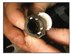
Remove the brake booster hose on the housing of the blower. The detail photos (middle and right) show you how to compress the two tabs on the bottom side of retainer and push the tabs out the side of the retainer housing to allow the retainer to be gently pulled off the flanged fitting attached to the blower housing.
