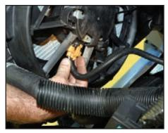
Plug in the electrical connector for the fan power by pushing it on the fitting on the fan assembly.
