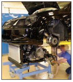
The first step is to get the engine located properly forward and aft so the radiator doesn't hang up on the front sheetmetal of the vehicle.
