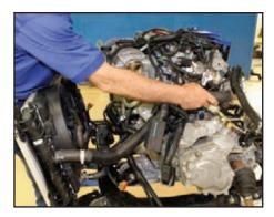
Route the long upper radiator hose around the side of the engine (over the transmission) to the fitting on the coolant distribution block near the cylinder head.
