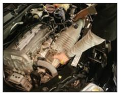
Carefully lift the supercharger out of the engine bay making sure nothing falls down into the opening in the intake manifold. As the blower comes off the intake, maneuver it toward the driver's side of the vehicle to clear the radiator hose.
