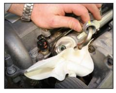
Place a rag around the fuel line fitting to absorb any excess fuel coming out of the rail. Running the engine with the fuel pump relay out of the fuse block should have bled off most of the fuel pressure, and the rag will absorb any remaining fuel.
