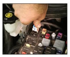
Install the "white" connector for the electronic power steering in the rear corner of the midplate of the fuse box. Push down on it until the lock tab "clicks". As a rule, if the "Service Power Steering" code lights up during startup, check this connection.
