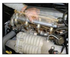
Install the fuel rail with the fuel injectors loaded on it into cylinder head. Carefully push down on the fuel injector rail until the rail mounts seat close to the cylinder head mounting bosses.
