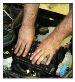
With all the connectors situated properly in the midplate, push down firmly to seat the connectors in the midplate.
