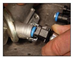
Line up the tangs in the fuel rail with the grooves in the injector clip to install them correctly.
