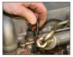
Reinstall the coolant temperature electrical connector on the sensor that is located on the cylinder head by pushing it onto the sensor mounted to the head. It will "click" when the lock tab is fully seated and will not pull off without depressing the tab.
