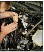
Use the awl to persuade the upper engine mounts to line up with the threaded holes in the body. Hand start the threads on the 16 mm mount bolts.
