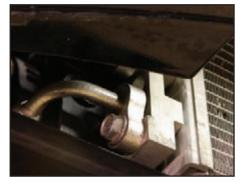
Tighten the 13 mm holddown bolt for the A/C fitting to 15 in-lbs (20 N-m).
