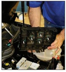
This photo shows you the bottom of the fuse box "midplate" that needs to be carefully installed over the various connectors. You'll need to finesse the connectors around to get them to "seat" in the connections that are molded into the bottom of this plate (shown in the photo).
