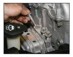
Hand start the three 16 mm upper engine mount bolts into their threads.
