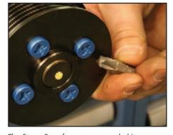
The Stage 2 performance upgrade kit comes with a special tool to tighten the hub/pulley bolts.
