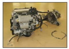
In the last chapter, we showed you how to get the engine out of the 2005-2007 Chevrolet Cobalt SS Supercharged vehicle and separate the engine and transmission. A 2004-2007 Saturn Ion Red Line would be similar. This chapter will show you the details necessary to reinstall these assemblies into the vehicle.
