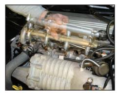
Flip the fuel rail over to prep to reinstall.
