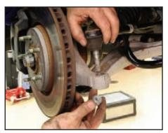
Wipe off the shaft of the steering tie rod and push it firmly into the tapered hole in the spindle upright.
