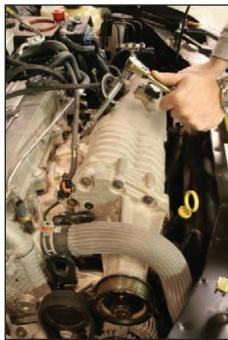
Remove the four 6 mm bolts holding the supercharger onto the intake manifold. There are two little black plastic "guides" that nest in the top of the supercharger bolt holes. Make sure these don't get lost as you'll need them to reinstall the blower.
