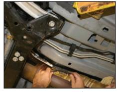
Reinstall the electrical connector for the O<sub>2</sub> sensor until the lock tang "clicks" in place.
