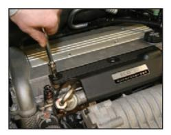
Unbolt the "Ecotec" engine cover by removing the two T30 Torx bolts.
