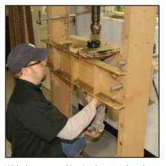
With the press making its downward stroke pushing the shaft out of pulley, be prepared to "catch" the supercharger when it comes free of the stock pulley.
