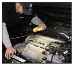
Check for leaks at the fuel lines. If there are any leaks, inspect to make sure the mating points are properly aligned and threaded on. If they are, retorque the fittings and reinspect with system under pressure. If everything is dry, crank the engine until it starts. Let it run while you check the fuel rail again for leaks.
