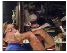
Push the lower A-arm up to seat the ball joint shaft in the spindle upright. Slide the 15 mm lock bolt through the upright from the rear to the front to hold the ball joint in place and hand start the 16 mm nut on the bolt.
