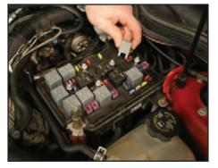
Pull out the fuel pump relay while engine is running to bleed off fuel pressure.
