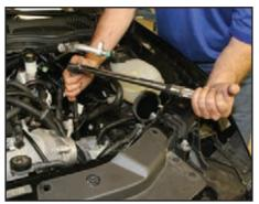
Torque the upper transmission mount bolts on the driver's side to 74 ft-lb (100 N-m).
