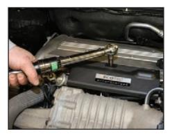
With the engine inspected for leaks and deemed sound, install the engine cover onto the engine, hand start the two T30 Torx engine cover bolts and torque them to 89 in-lbs (10 N-m).
