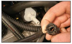
Remove the evaporator-purge hard line fitting by rotating the tab downward on the fitting to unlock it from the nipple on the solenoid. Take a look at the photo on the right to see how the fitting locks on the nipple.
