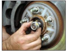
These are the hub washer and 30 mm lock nut that need to be hand started on the axle threads.
