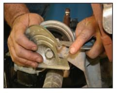
Slide this heat shield on the rear engine mount bushing before installing the 18 mm bolt.
