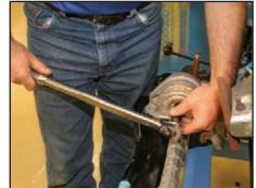
Hand start the threads on this rear engine mount bushing bolt and torque it to 74 ft-lbs (100 N-m).
