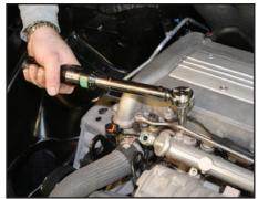
Hand start the threads of the coolant steam pipe bolt and washer into the cylinder head.
