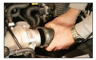
Start removing the hose by pushing it off the throttle body flange as shown.
