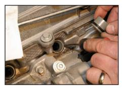
The fuel injectors seat into plastic "inserts" in the cylinder head—these inserts should remain in the head but sometimes stick to the fuel injectors when they are removed. If the inserts come out, reinstall them into the head after wiping a light coat of Vaseline on the O-ring seal.
