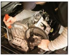
To get the belt on the crank pulley, it usually works best to use a long screwdriver or pry bar to lightly maneuver the belt onto the big crank pulley while lightly wiggling the belt in your other hand. This is tight and your vision into this space is limited, so be patient!
