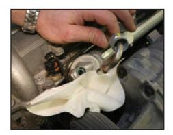
Some fuel will leak out of the fuel rail after it is loosened and removed, so place a rag around/underneath the fitting to catch this fuel.
