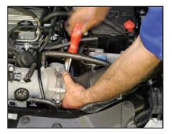
Tighten the adjustment bolts on the hose clamps at each end of the inlet tube to 1/8-turn past hand tight. Do not overtighten this hose, as it will collapse the induction tube.
