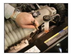
Remove the two 10 mm bolts that hold the coolant reservoir for the intercooler.
