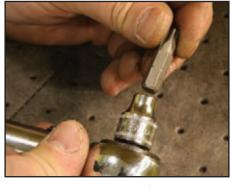
Place the Stage 2 hub/pulley fastener tool into an 8 mm socket on a large ratchet to tighten the bolts in a radial pattern.
