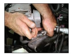
Tighten this 13 mm bolt to 15 ft-lbs (20 N-m).
