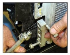
Install the top one of the two A/C fittings that go on the side of the A/C condenser. Apply a light coat of Vaseline to the O-ring on the fitting and push it into the condenser. The other fitting is plumbed into the vehicle, so it will be installed after the engine is reinstalled in the vehicle.
