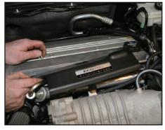
If no leaks are found, shut the engine off and install the engine cover with the two T30 Torx.
