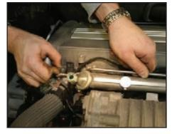
Position the steam pipe in place in front of the cylinder head.
