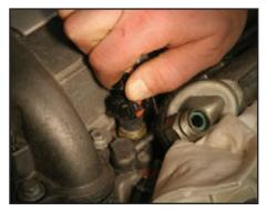
Remove the temperature sender electrical connector on the cylinder head by depressing the lock tab on the wire end of the connector and pulling up.
