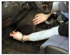
The first step in removing the fuel injectors is bleeding off the fuel pressure in the fuel rail. This is accomplished by removing the relay controlling the fuel pump from the fuse block. On the Saturn Ion Red Line, the fuse block is located under the center stack of the dashboard.
