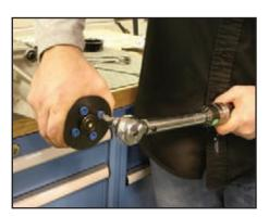
These fasteners will be torqued once the blower is back on the vehicle and the belt is holding the pulley in place, so just get the fasteners hand tight and move on to the next step.
