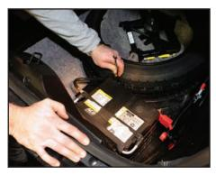
Loosen the 10 mm (5/16" on Ion) nut on the battery cable and wiggle the cable off the battery stud. Wrap the cable end with a rag and place it on the floor.
