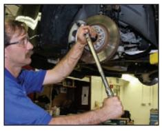
With a helper holding the brake pedal down firmly, torque the drive axle nuts to 37 ft-lb (50 N-m), back them off 3/4-turn, then retorque to 37 ft-lb (50 N-m) and rotate another 30 degrees.
