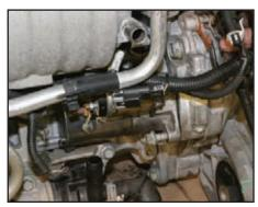
Install the starter and hand start the two 15 mm bolts. Tighten them to past hand tight and torque to 30 ft-lb (40 N-m).
