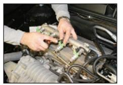
Start to remove the electrical connectors on each stock, green fuel injector. For more on how to perform this activity, refer to the sidebar "Removing electrical connectors from fuel injectors" on the top of the next page.
