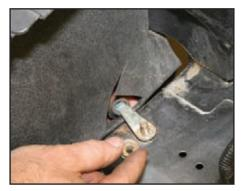
Feed the ground cable through this opening and onto this bolt/stud. Tighten the 13 mm nut onto the stud and torque to 18 ft-lb (25 N-m).
