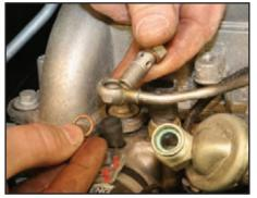
Pivot the steam pipe back over the front of the engine in preparation for reinstalling the steam pipe bolt.
