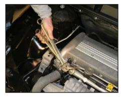
Unbolt the fuel line fitting by loosening the 24 mm fuel line nut. Use a 21 mm wrench to pull on to avoid damaging the fuel rail. Be careful as some pressurized fuel might spray out when this fitting is loosened, so cover the fitting with a rag as it is loosened.
