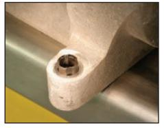
This is one of the two black plastic guides that nest in two of the bolt holes on the blower. Be careful to not let these drop into the intake upon supercharger removal. They hold the supercharger bolts.
