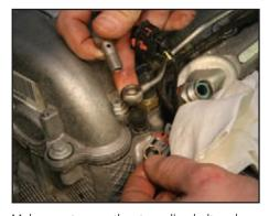
Make sure to save the steam line bolt and washer for reinstallation.
