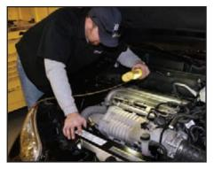
Check your work for any leaks in the fuel system, coolant system (at the steam pipe) and any other areas you disassembled. Make sure all electrical connections are firmly on their mating points and all tools have been removed from under the hood.
