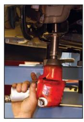
If you can, use an air impact gun to tighten the cradle bolt holes to a very tight setting so you can lift the vehicle up before doing the torque wrench check on the bolts.
