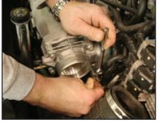
You can either disconnect the electrical connector on the bottom of the throttle body (not easy if you haven't done it before), or disconnect the four bolts holding the throttle body on the supercharger body. We'll show you the throttle body removal, as it is easier on your first Stage 2 install. To start, remove the four 10 mm bolts holding the throttle body on the supercharger.
