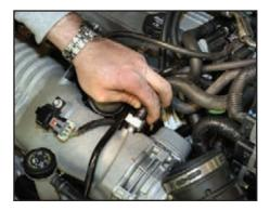
Install the brake booster line onto the side of the supercharger housing and push down on the white "C" clip lock to ensure that the line stays installed.
