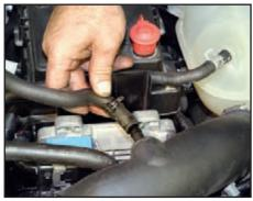
Install the EGR feed tube on to the nipple on the inlet tube.
