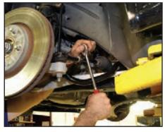
Tighten the lock nut to just past hand tight with a 13 mm deepwell socket on a 12-inch extension and ratchet wrench.
