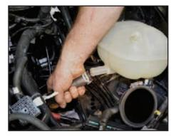
Pull the engine coolant system overflow tank up to the nipple on the overflow tank.
