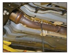
This is what the exhaust downpipe should look like when it is properly installed.
