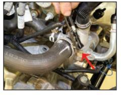
Using a pair of pliers (you see the business end of the remote pliers from Snap On, but in this case, you could use standard pliers), compress the hose clamp to slide the hose on the fitting. Release the clamp tangs to lock the hose in place on the fitting.
