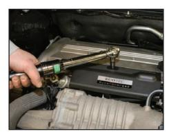
Torque the T30 Torx bolts to 89 in-lbs (10 N-m) and Install the Stage 1-supplied EO sticker over the stock engine sticker under the hood.
