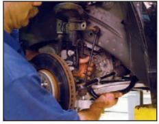
Lift up on the swaybar link in preparation for reinstalling on the strut mount.
