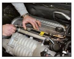
Position the fuel line onto the engine and hand start the fuel line fitting onto the fuel rail. Before threading this on, it is a good idea to wipe a light coat of Vaseline on the mounting interface of the fuel rail and inspect this fitting to make sure the two O-rings that seal this point are in place.
