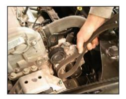
Even more exciting than removing the stock belt is weaseling the Stage 2 belt into the space between the big crank pulley and the front of the engine. Start by pinching the belt down like this when starting to push the belt into place over the crank pulley.
