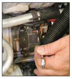
Install the big connector main power wire onto the large stud and tighten the 13 mm nut to 1/4-turn past hand tight.
