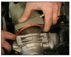
Reinstall the throttle body by first making sure the red O-ring seal in the supercharger flange is seated properly in its groove.
