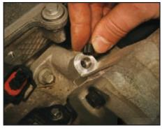
Make sure the two black plastic locaters that sit in the bolt holes are positioned properly to locate the blower bolts.
