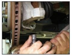
Now, install the ball joint into the spindle upright. To do this, the ball joint shaft will need to be maneuvered to align with the hole in the spindle upright.
