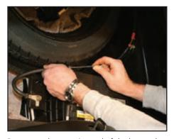
Reconnect the negative end of the battery by sliding the connector over the stud of the battery. Torque the 10 mm (5/16" on Ion) nut to 89 in-lbs (10 N-m).
