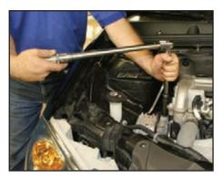
Torque the upper engine mount bolts on the passenger's side to 74 ft-lb (100 N-m).
