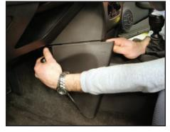
Pull the Red Line panel toward the rear of the vehicle to remove it from the center stack.
