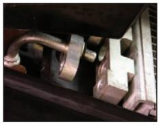
Up under the front fascia on the passenger's side, install the bottom of the two A/C fittings that go on the side of the A/C condenser. Apply a light coat of Vaseline to the O-ring on the fitting and push it into the condenser.
