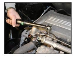
Hand start the two 10 mm bolts into the bosses and torque the fuel rail bolts to 89 in-lbs.
