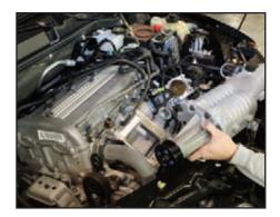
With the Stage 2 pulley installed, now it is time to reinstall the supercharger. To start, make sure the metal aligning pins are located in the intake manifold bolt holes and that the supercharger-to-intake-manifold gasket is seated in its groove. Also make sure the bypass seal is properly situated on the intake before installing the blower.
