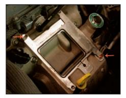
These two metal locating pins seat in the intake manifold (arrows) and have a tendency to stick to the blower housing. Make sure they don't fall down into the opening in the intake! If the pin(s) stay in the blower when it is pulled out, pull them out and reinstall them in the intake. Place some tape or a rag over the intake opening to minimize chances of something falling into the engine.
