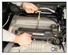
Move under the hood of the vehicle to start removing components to allow for the installation of the GM Performance Stage 1 performance upgrade kit. The first step is to unbolt the engine cover that is held in place with two T30 Torx screws.
