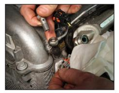
Remove coolant steam pipe on front-passenger side of engine with 14 mm socket. Make sure to save the copper washer below the 14 mm fitting, and once removed, it is a good idea to plug this hole with 1/4-inch rubber stopper to minimize coolant drooling out of the hole.
