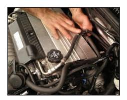
Place the fuel line in the plastic clip on the cylinder head and close the clip over the hose to lock it in place.
