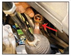
Lightly polish the end of the shaft that comes out of the rack and pinion unit with a scotchbrite or steel wool pad to knock off any rust or dirt particles in preparation for sliding the steering U-joint on the shaft. This shaft has been prepped already.
