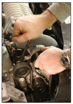
Now is the time to install the Stage 2 belt on the Stage 2 equipped supercharger. To start this step, make sure the belt is fully installed on all the pulleys—especially the air conditioning pump pulley as this often will become misaligned during the belt reinstall process. Compress the tensioner with a 15 mm open end wrench while working to string the belt back over the tensioner pulley.
