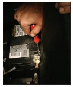
In the trunk, install the battery cable, start the vehicle and start checking for leaks, loose hoses and any other "issues". Top off the coolant mix before closing the hood and enjoying a drive in your newly reassembled Cobalt SS Supercharged.
