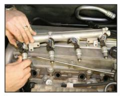
Carefully install the fuel injector electrical wiring connectors onto each fuel injector. Each connector from the wiring harness really will only reach the correct fuel injector, but for our more talented enthusiasts, make sure the No. 1 cylinder connector is attached to the No. 1 fuel injector. Also, make sure the connector is fully seated on the fuel injector-a loose connection will cause the engine to light up the 'check engine' light.
