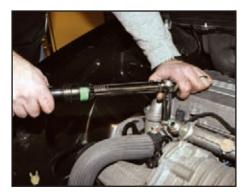
Torque the steam pipe bolt to 89 in-lb (10 N-m).
