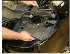
Reinstall the closeout panel that is positioned above the air cleaner box.
