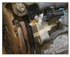
Use a few pieces of masking tape to hold the shim in place on the engine block.
